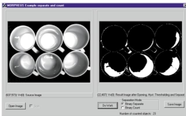
Most image analysis problems are very complex and can only be solved by combining a number of basic transformations. It is therefore possible in Morpheus to execute an unlimited number of consecutive transformations; the output image of one operation becomes the input image of the next one. In this way, it is possible to program very powerful image analysis procedures specifically for a particular problem within a very short space of time.
