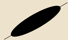
Object with pronounced orientation showing the axis of the minimum moment of inertia.
